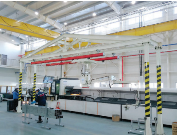
Laser Processing System Equipment that precisely cuts tube lengths and processes holes in round and square tubes using a high-power laser system. Features - Enables high-speed, precision cutting - Supports processing of various materials, including steel and aluminum - Capable of machining complex shapes and patterns - Minimizes material deformation through a non-contact processing method
